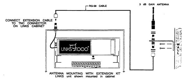
cabinet. Secure the antenna to the TNC connector mounted on the Extension Kit Mounting Bracket.
